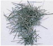
Fig -1: Straight Steel Fiber
