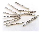
Fig -2: Crimped Steel Fiber
