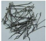
Fig -3: Hooked Steel Fiber
